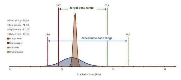
The figure shows the process and release specifications in relation to the statistical distribution of the measured dose at the routine monitoring position. The correlations and derivations of the different values are shown below:
